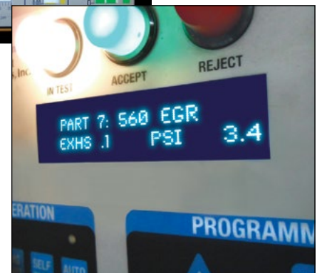
Final Pressure testing to O.E. Specifications
